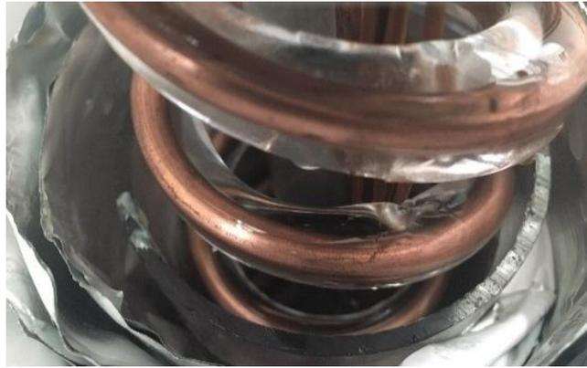
**Figure 8. Image of the inside of the small-scale prototype DPUBT showing ice formed on the heat exchanger in the inner tank when the coolant at  $-2\text{ }^{\circ}\text{C}$  was used to charge the DPUBT.**
